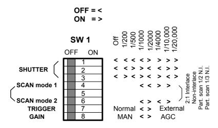
Fig. 18. Switch settings for switch on rear
